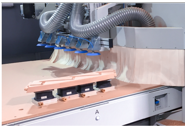
Adapter-Plates AP-G with vacuum block VCBL-B when clamping a wooden workpiece
